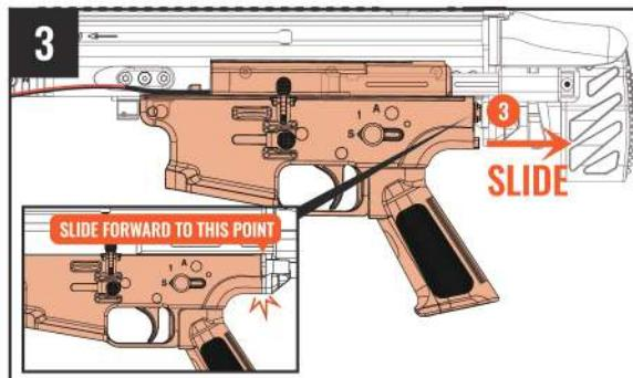
Push lower receiver backward to lock position and insert takedown ping.
