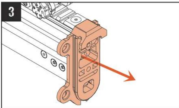
Remove rear sling swivel hinge.
