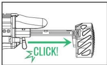
After adjusting the buttstock, please make sure that the buttstock adjustment latch has been properly locked to the position.
