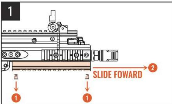
Remove the 2 screws of the lower rail, and slide the lower rail piece forward to remove it.
