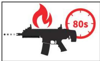
Please do not continue to operate for more than 80 seconds to avoid battery and motor overheating problem, resulting in the risk of combustion.
