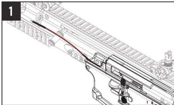
Make sure the wire position as shown in diagram when assemble upper & lower receivers.
