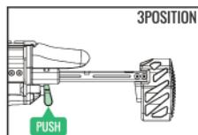
Press and hold "STOCK LEVER" to pull out the stock, SCAR SC STOCK has 3 positions that can be adjusted.
