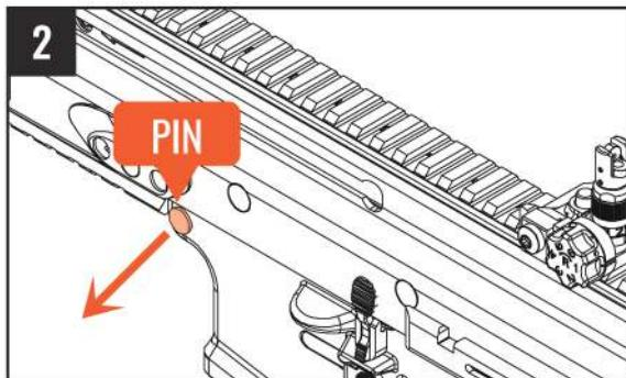
Remove the pin from the gun body.
