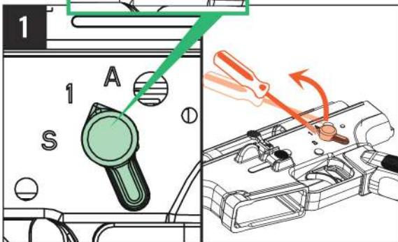
Adjust the selector to the middle of SAFE and SEMI, and use a flat-head screwdriver to gently lift up the selector from its top edge.
