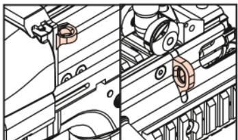
There are strap buckles on the left and right sides under the front sight & in front of the buttstock to install the gun strap.
