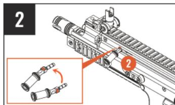
Rotate the handle upwards until the cut surface is facing up.
