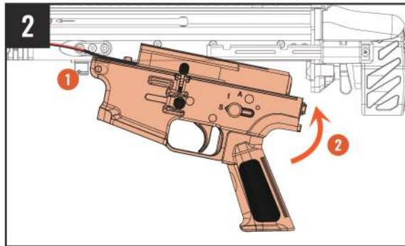
Follow the steps in diagram to assemble upper & lower receivers.
