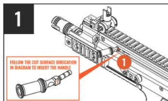
When installing the charging handle lever, follow the direction in Step 1 to insert the handle.
