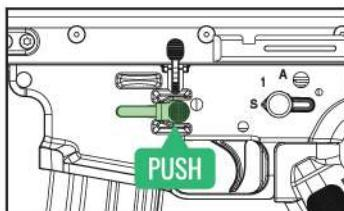
SCAR SC is equipped with ambidextrous magazine release button, press and hold the magazine release button to remove the magazine.
