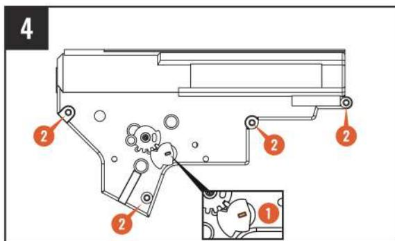
Remove the pin in Step 1, and the 4 screws in Step 2 in the order to disassemble the box.
