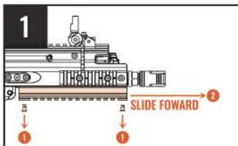
Remove the 2 screws of the lower rail and slide the lower rail forward. After installing the 3-piece (10cm length) battery, please store the wire properly, and then install the lower rail back in order to lock the screw.
