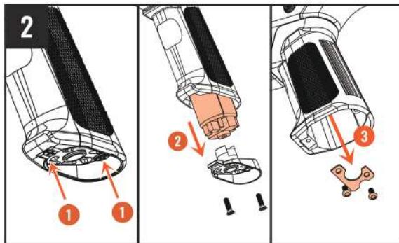
The motor can be removed after removing the marked screws and the motor grip plate.
