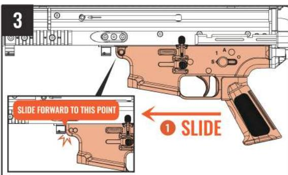
Remove the PIN of the lower body and push the lower body forward about 3cm to remove from the upper body.
