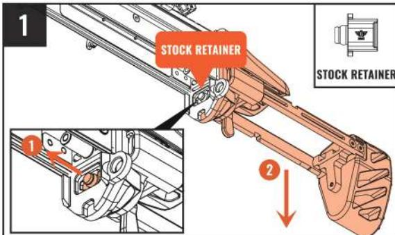
Press and hold the stock lever to pull the stock to full rear and then remove the stock retainer to separate the upper body from the rear stock.
