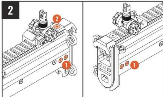
Remove the left & right 2 screws & the upper screw to remove the stock end plate.
