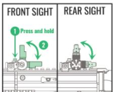
Adjust the front sight and rear sight according to the positions marked in the image.
