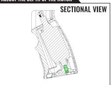
There is a stopper (green) on the bottom of the motor bottom cover. Use a 3.0mm hexagonal screwdriver to lock it up and down.
