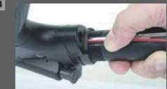
The wire should be held down tightly within the wire path when taking the wire.
