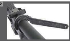
Before removing the stock tube lock, make sure that your ar-15 wrench is aligned properly before unscrewing the stock tube lock.
