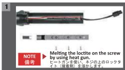
Remove the stock tube cover and the wire cover by removing the screws.
