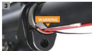
**WARNING** ► SHARP EDGES MAY CAUSE DAMAGE TO THE WIRE SET.
