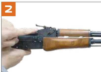
Press sight release latch and move forward and back to adjust.
