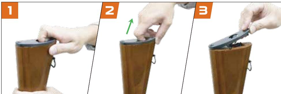
Push finger inside the moveable butt-plate and just pull back to remove the fix-stock end cover.
