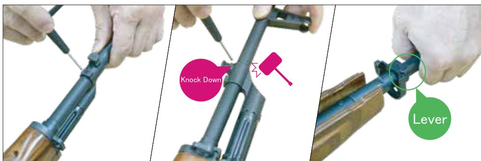
Remove hexagon socket screws (M4x5) then knock down the pin button and pull out the gas tube, unlock the front handguard cover lock and then take out the lower handguard cover.
