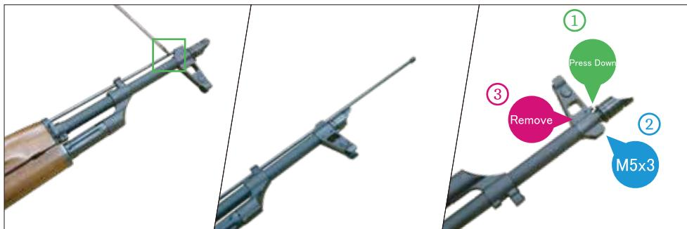
Remove the screw under the sight base, and also the cleaning rod.
